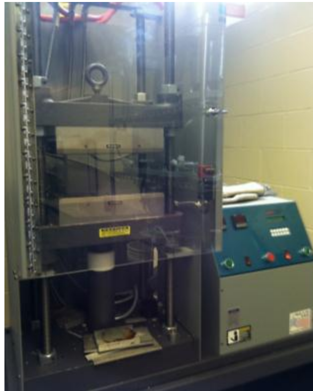
Figure C.4 Carver, Inc. compression molder (model 3893.4PR1A00).
